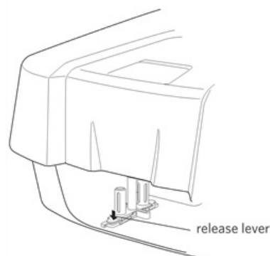
1. Pinch release lever and gently lower sample holder.
