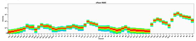
Spectral signature of cFluor® R685 from a Cytek® Aurora 5 laser system equipped with 355, 405, 488, 561 and 640 nm lasers using CytekAssaySetting.
