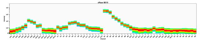
Spectral signature of cFluor® B515 from a Cytek® Aurora 5 laser system equipped with 355, 405, 488, 561 and 640nm lasers using CytekAssaySetting.
