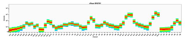
Spectral signature of cFluor® BYG781 from a Cytek® Aurora 5 laser system equipped with 355, 405, 488, 561 and 640 nm lasers using CytekAssaySetting.
