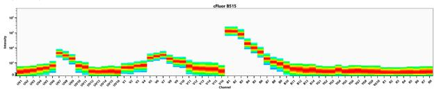
Spectral signature of cFluor<sup>®</sup> B515 from a Cytek<sup>®</sup> Aurora 5 laser system equipped with 355, 405, 488, 561 and 640 nm lasers using CytekAssaySetting.
